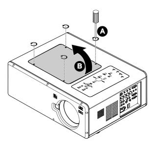
2. Loosen the two captive screws on the lamp module (A). Lift the module handle up as shown (B).
